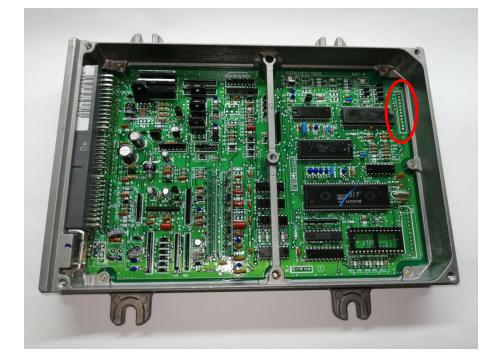
Remove the Board from the ECU Chassis and desolder all 12 Solder joints of FC1.
