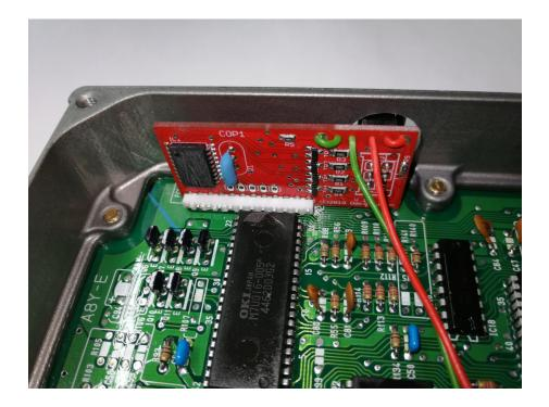
Finally solder the GREEN Wire to the ECU Connector A21 and the RED Wire to A25.
