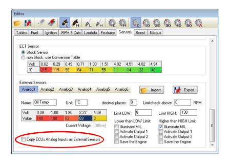
Make sure that the "Copy ECUs Analog Inputs as External Sensor" checkbox is UNCHECKED!
