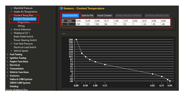
Enter Voltage to Temperature curve or Load from File. You can download our Coolant Temperature calibration from our website.
