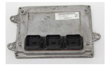
The Installation is easy by just connecting 3 wires: Green = SNET5V = to Pin A44 Black = GROUND = to Pin A9 (alternative A34, A35) Red = +5 Volt = to Pin A19 (alternative A24, A25)
