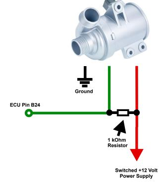
Connection to a ECU with HIGH SIDE DRIVER Output: (Automatic ECU)
